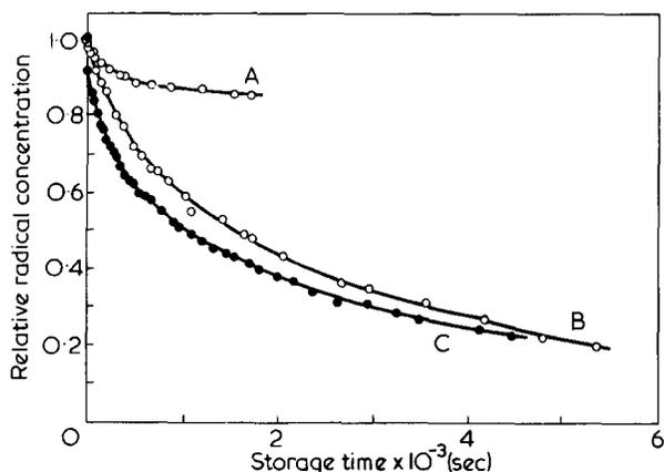
Figure 9 The decay curves of alkyl radicals in irradiated urea-polyethylene complex and that of polyethylene single crystal. A, 380K; B, 411K; C, 327K. ○, Relative concentration of free radicals in urea-PE complex; ●, relative concentration of free radicals in solution grown PE single crystals
