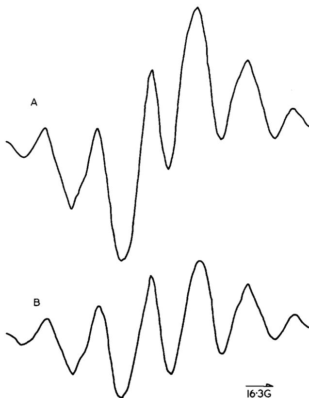
Figure 6 E.s.r. spectra of irradiated polyethylene single crystals. Observation was made at liquid nitrogen temperature after irradiation at the same temperature. A, observed after heating up to 195K for a long time; B, spectrum after heat treatment at 269K for 280 min
