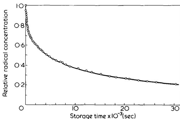
Figure 1 The decay curve of alkyl radicals trapped in irradiated polyethylene single crystals, A-85, at liquid nitrogen temperature after heating to 273K for a long time. Experiments were made at 307K. —, shows calculated decay curve of equation (7); the constants in equation (7) are:  $A = 1.2 \times 10^{-2} \text{ (sec}^{-1/2}\text{)}$ ;  $B = 4.5 \times 10^{-5} \text{ (sec}^{-1}\text{)}$
