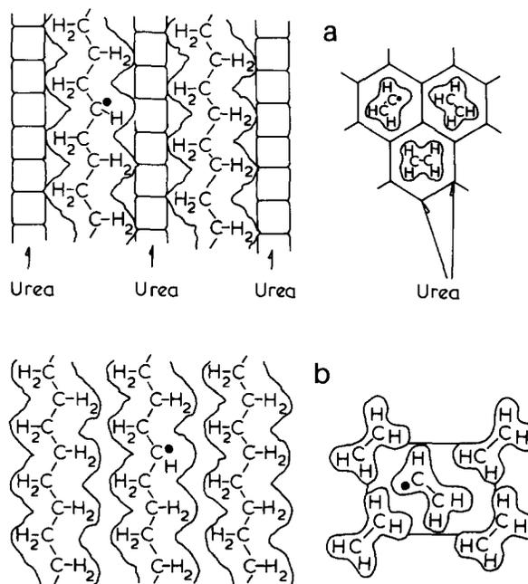
Figure 10 Schematic model of (a) urea-polyethylene complex structure and (b) polyethylene single crystals
