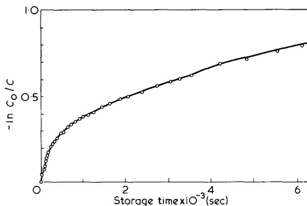
Figure 3 Logarithm of inverse concentration of alkyl radicals vs. duration of time of storage at 307K
