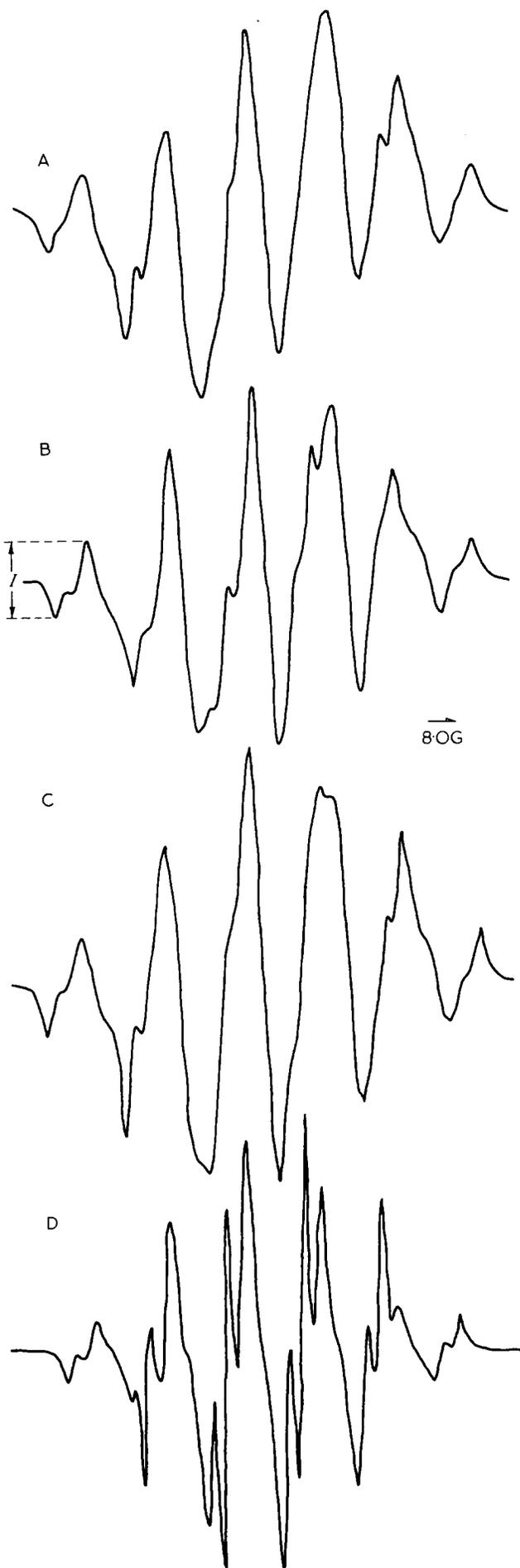
Figure 8 E.s.r. spectra of alkyl radical produced in polyethylene single crystals (A, B) and urea polyethylene complex (C, D). A, 77K; B, 280K; C, 77K; D, 289K
