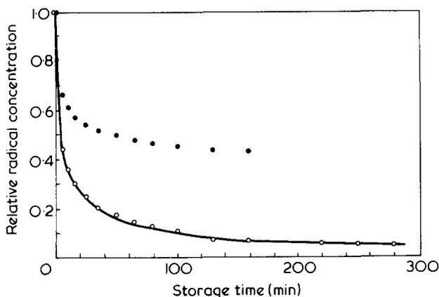
Figure 5 The decay curve of alkyl radicals trapped in irradiated polyethylene single crystals A-85 at 269K after heating at 195K for a long time. Irradiation was made at 77K and e.s.r. observations were made at 77K.  $\circ$ , Show the reduced amount of decay obtained after subtracting the amount of non-vanishing radicals. —, shows calculated decay curve with  $A = 4 \times 10^{-2} \text{ (sec}^{-1/2}\text{)}$  and  $B = 1 \times 10^{-3} \text{ (sec}^{-1}\text{)}$
