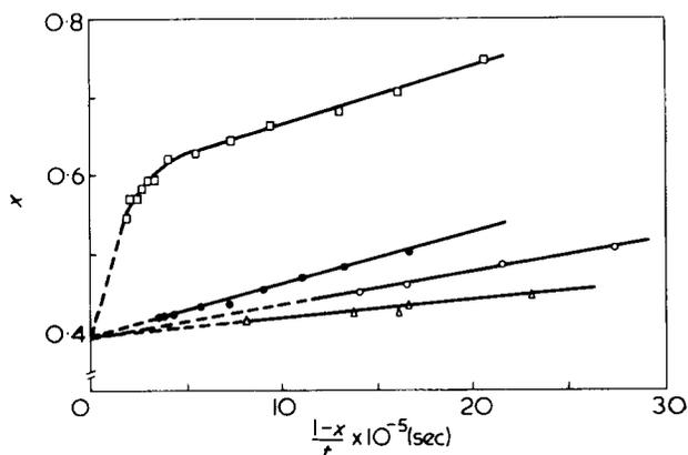
Figure 7 The relative concentration of alkyl radicals vs. value of  $(1-x)/t$  at various temperatures:  $\square$ ,  $-23.0^\circ$ ;  $\bullet$ ,  $-8.0^\circ$ ;  $\circ$ ,  $-3.0^\circ$ ;  $\triangle$ ,  $-1.5^\circ$  C. E.s.r. measurements were made at 77K
